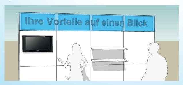
In case of backlit panels, please note that about 1 cm is not illuminated all around because the magnetic tape runs at these points. This information must be considered for layout purposes. As a consequence, the motif/text must be put away from the edge.
